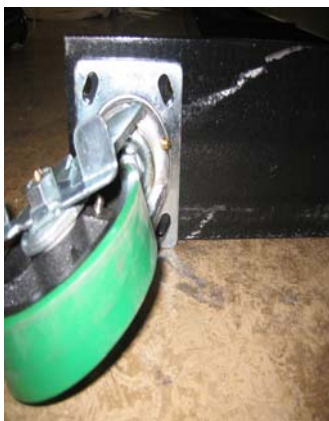
WRONG plate direction
