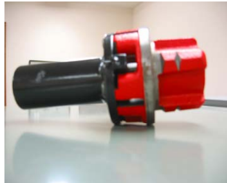
Die Head which fits in power winder
