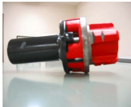
Die Head which fits in power winder
