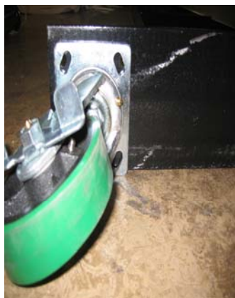
WRONG plate direction
