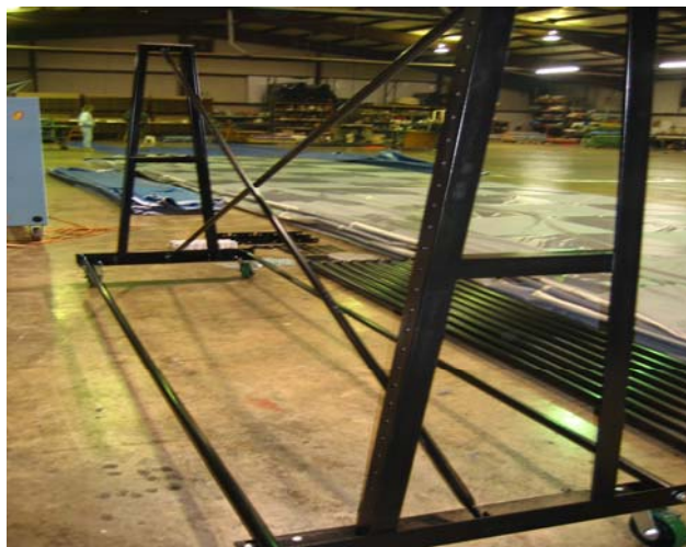
Both Spacer tubes and cross braces attached to A-Frame ends.
