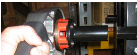
Adaptor fits onto power winder
